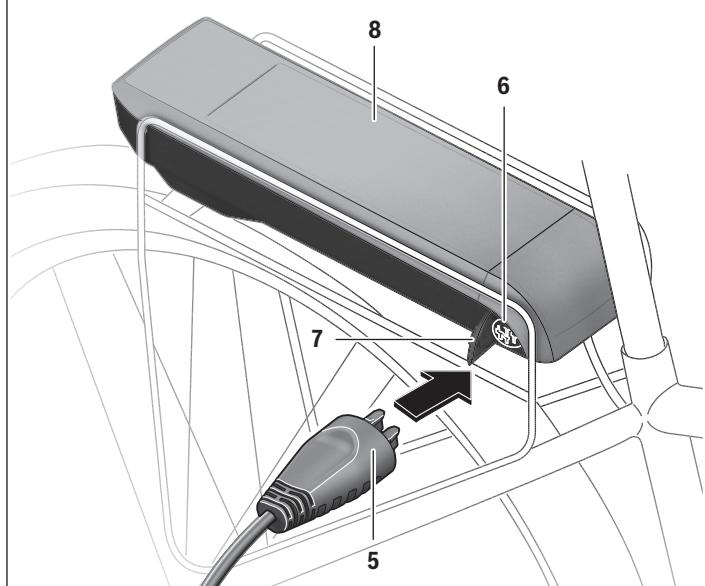
Switch the battery off. Clean the cover of the charge socket **7**. In particular, prevent the charge socket and the contacts from getting dirty, e.g., with sand or soil. Lift the cover of the charge socket **7** and plug the charge connector **5** into the charge socket **6**.
