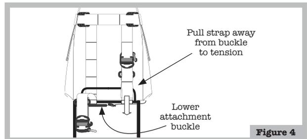
5. On the underside of the rack, attach the buckle ends together. The buckle will make a noticeable “click” when properly installed (Figure 5). Tension the strap by pulling the end of the strap away from the buckle. A loop is sewn into the end of the strap so a finger can be inserted for additional leverage (Figure 6). Appropriate tension will help assure the bag remains stable while riding.
